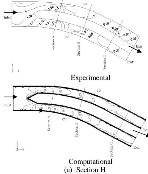
Fig. 4. Comparison of normalized velocity distribution at Section H obtained through Computational and Experimental investigation
