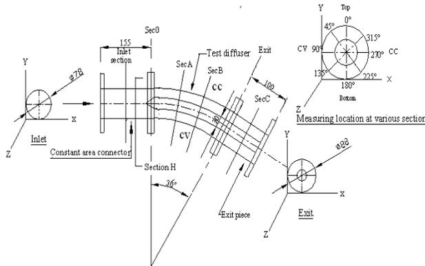
Fig.1 Geometry of test diffuser and measuring locations
