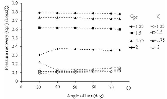
Fig.7. Variation of mass average pressure recovery and loss coefficients.
