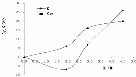
Fig. 3. Variation of mass average pressure recovery and loss coefficients
